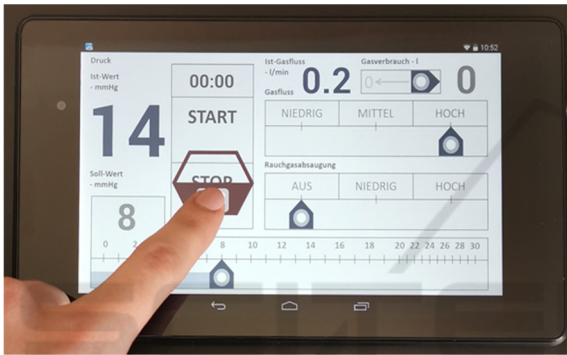
Figure 2: Test interface of the slide control elements for the adjustment tasks with electro-tactile feedback.
