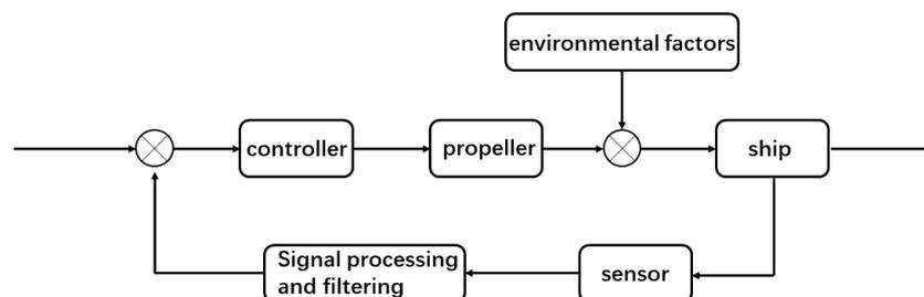
Figure 1: The structural diagram of the ship's dynamic positioning system.
