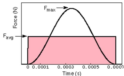
Figure 4: Example of a Force-Time function of a collision (Russell 2011).
