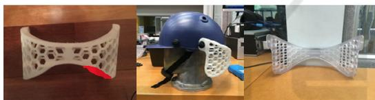
Figure 12: 3D printed neck protection guard.
