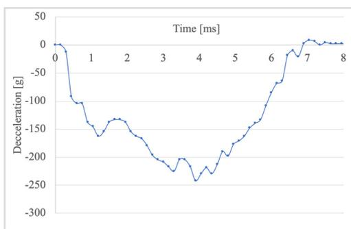
Figure 11: The deceleration of cricket ball impacting NPG.
