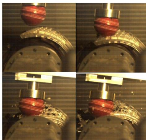
Figure 13: High speed camera images of the cricket ball impacting the 3D printed neck protection guard.
