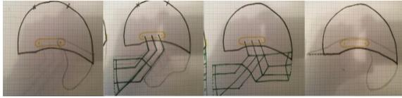
Figure 3: Conceptual sketches of the neck protection guard.
