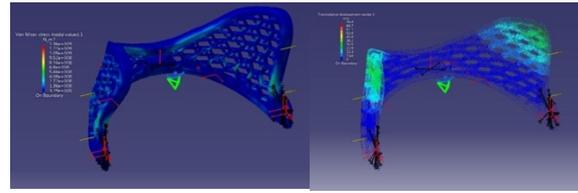
Figure 9: Stress distribution of honeycomb design under static loading conditions.
