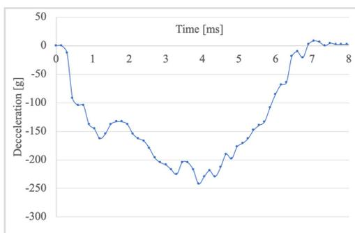
Figure 11: The deceleration of cricket ball impacting NPG.
