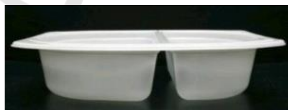
Figure 1: The size of two holes plastic tray 118x179x40 mm with layer structure is PP/PP + Additive/Tie/EVOH/Tie/PP + Additive/PP.
