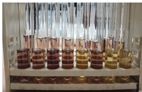
Figure 1: Testing the antioxidant activity of liquid smoke of cocoa pod skin DPPH method.
