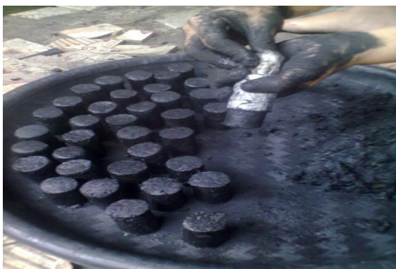
Figure 5: Process of Durian leather briquette printing
