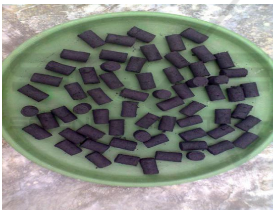
Figure 6: The drying process of durian leather briquette
