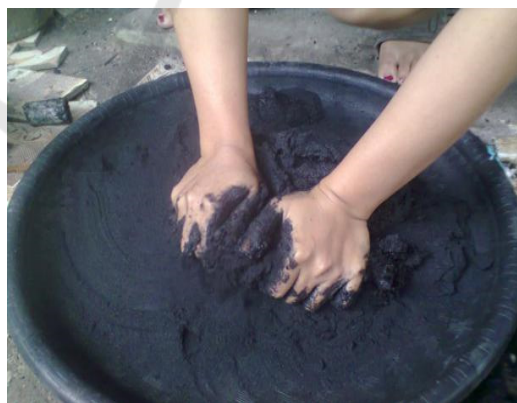
Figure 4: Process of mixing adhesive and powder
