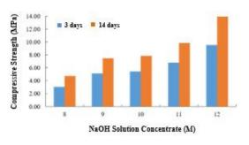
Figure 5: Graphic of NaOH solution concentrate on compressive strength (Writer, 2019)
