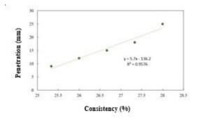
Figure 3: Graphic of normal consistency on cement paste (Writer, 2019)
