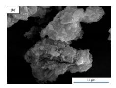
Figure 1: SEM of FA (100 wt%) with magnification value of (a) 250x and (b) 10.000x (Writer, 2019)
