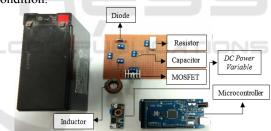
Figure 3: Hardware implementation of the circuit on the buck-boost converter system.
