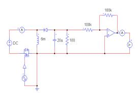
Figure 2: PSIM simulation circuit on the buck-boost converter system.
