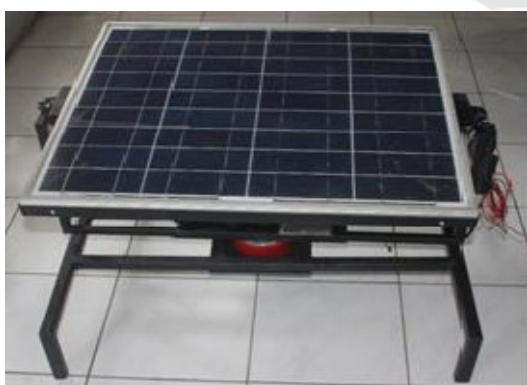
Figure 3: Mechanical Design for solar Tracking
