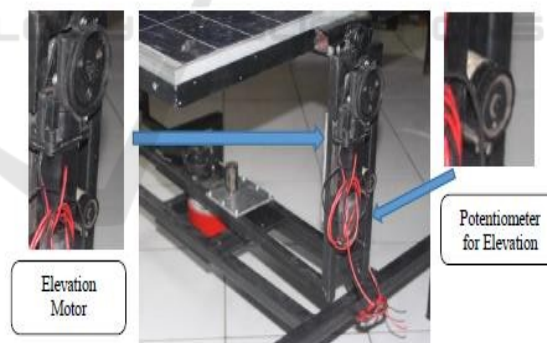
Figure 5: Mechanical Design of Solar tracking-elevation motor.
