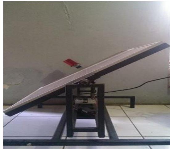
Figure 8: Position of solar panel with -30^{\circ}\text{C} from standard elevation
