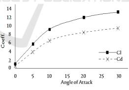
Figure 8: Cl and Cd v Angle of Attack
