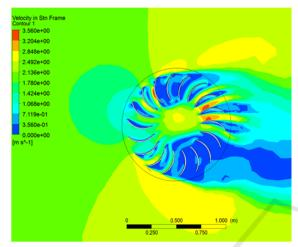
Figure 7. The flow contour of the cross-flow wind turbine
