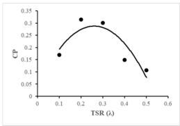
Figure 6. Data of power coefficient versus TSR
