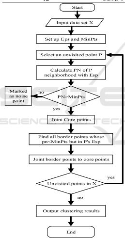
Fig 3. Process of DBSCAN clustering algorithm.
