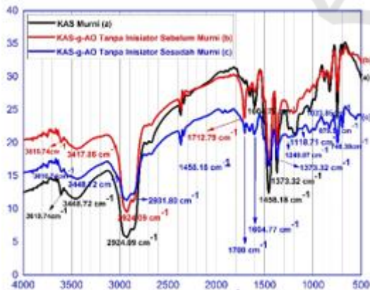
Figure 1: Spectrum of CNR-g-AO FT-IR without DKP Initiator.
