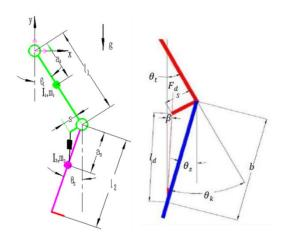
Figure 3. Dynamics model of lower limb prosthesis.
