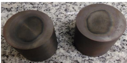
Figure 1: Unjoined specimen ( T_w=950^{\circ}\text{C} , t_w=60\text{min} , P_w=10\text{MPa} ).
