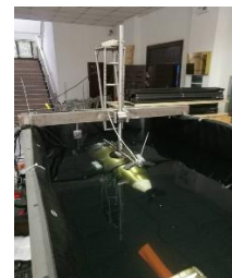
Figure 8. Physical drawing of thrust test device.
