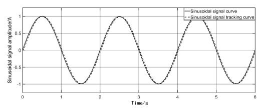
Figure 7. Sinusoidal signal tracking curve
