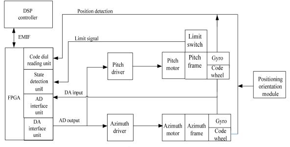
Figure 3. Schematic diagram of servo control circuit.
