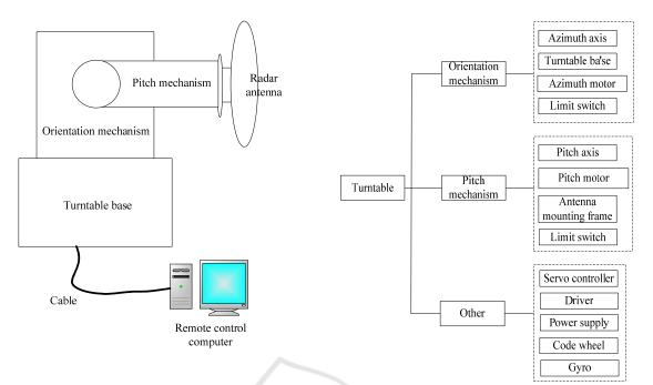
Figure 1. Block diagram of the stable platform.
