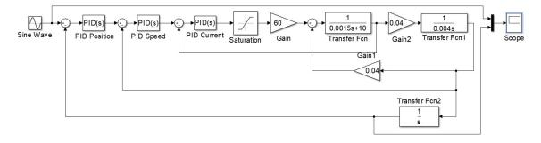
Figure 6. Sinusoidal signal tracking simulink simulation model
