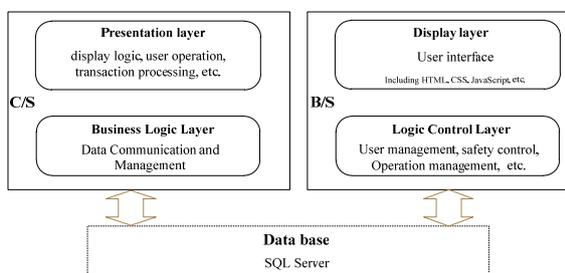
Figure 2. Software structure of the cloud platform.
