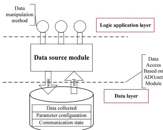
Figure 3. Data source module of C/S.
