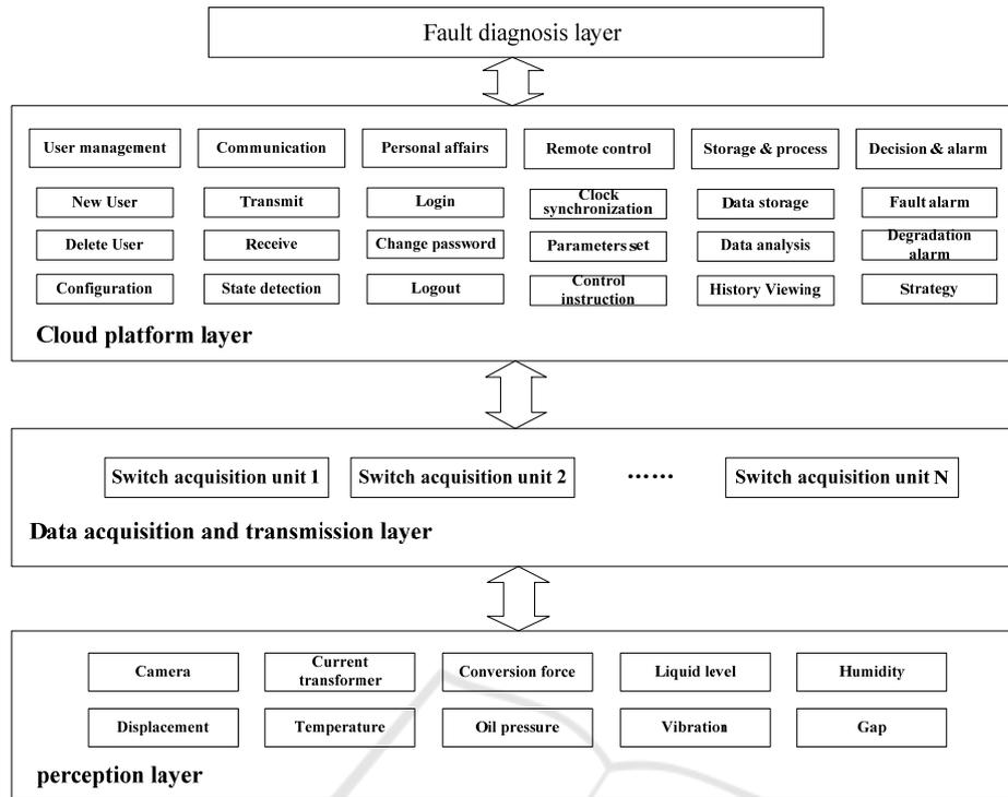
Figure 1. Structure of the fault diagnosis and PHM system for switch equipment.
