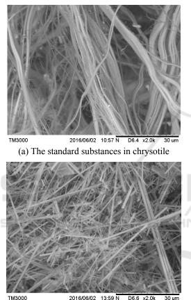
TM3000 2016/06/02 13:59 N D6.6 x2.0k 30 (b) The standard substances in amosite
