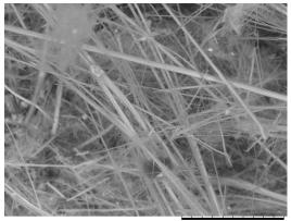
TM3000 2016/06/02 11:40 N D6.4 x2.0k 30 um (c) The standard substances in crocidolite
