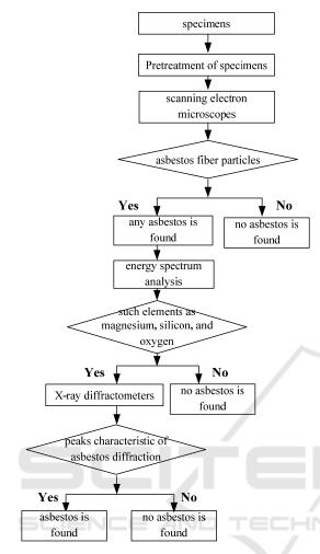
Figure 1. Determination procedures with scanning electron microscopes and X-ray diffractometers.
