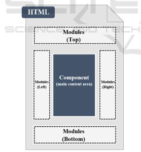
Figure 3: Template of a page in Joomla!-based Web applications.
