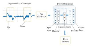
Figure 2: Deep autoencoder feature extraction approach (Acc represents acceleration signal).
