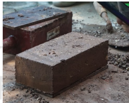
Figure 13. Wet soil and sawdust block
