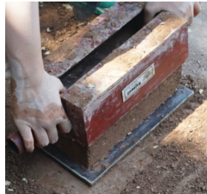
Figure 12. Taking the mould process
