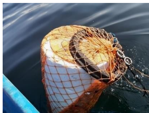
Figure 7: Fishing Net Disturbing The Buoy of ADCP.
