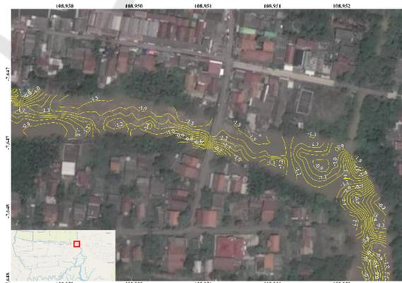
Figure 6: Bathymetry in research location -> LLWS=0.
