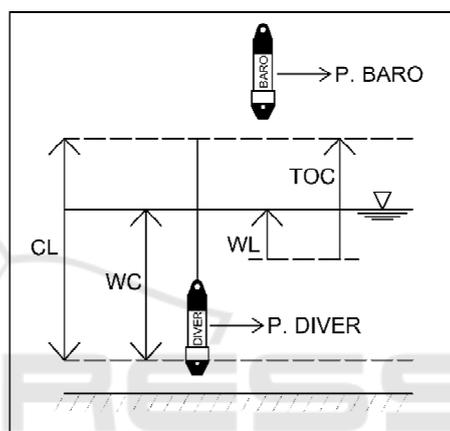
Figure 1: DIVER installation scheme.
