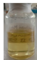
Figure 6: Product methyl esters of transesterification castor oil catalyzed by mesoporous silica CaO impregnation (MS 8.4Me CaO).
