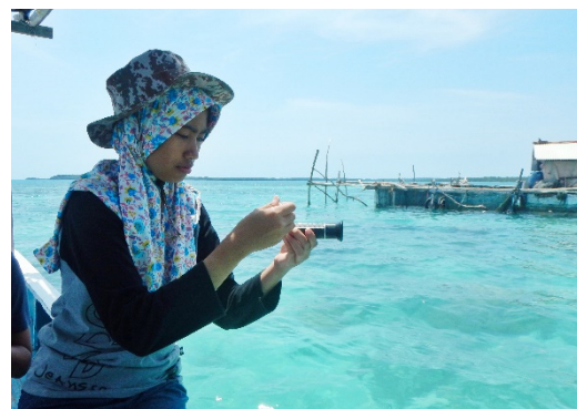
Figure 4: Water Quality Measurement using Refractometer for Salinity.
