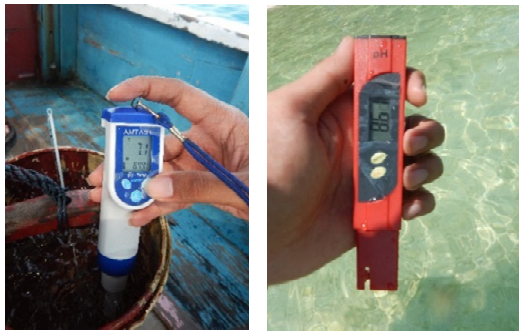
Figure 5: Water Quality Measurement using DO meter and pH meter.
