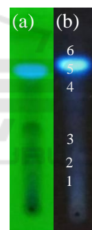
Figure 1. TLC profile of ethyl acetate fraction (Ds-II) after being developed with chloroform : ethyl acetate : methanol (7:2:1) as mobile phase. TLC plate were visualized under UV light at wavelength (a). 254 nm and (b) 366 nm.
