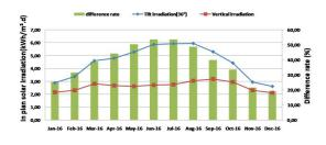
Figure 3: Monthly average daily irradiation respectively on the vertical plan of the PV array and on the optimal angle for the site (36°).
