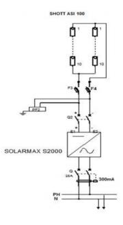
Figure 2: Diagram of the 2.4kWp a-Sigrid connected
