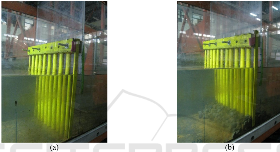
Figure 4: CPB: a. CPB without bottom protection a. CPB with bottom protection.
