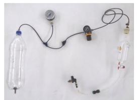
Figure 3: Components of pressurized air tubes.
