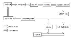
Figure 5: Fuel delivery scheme in electronic fuel pump system.
