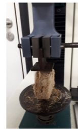
Figure 3: Position of the rice straw briquette in the compressive test.
