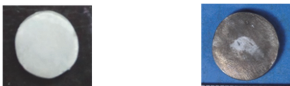
Figure 4: Image of macrostructure aging treatment material (left) before corrosion test (right) after corrosion test.
