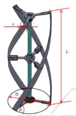
Figure 9: Gorlov Helical Turbine with 135° foil (Akimoto et al., 2013)
