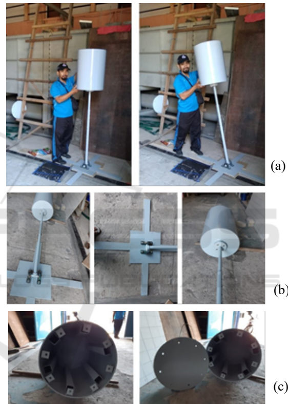
Figure 3: Physical model of AT-OWEC main structure.
