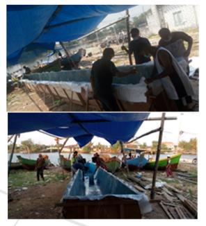
Figure 6: FRP Lamination Process.
