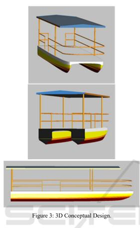
We can see in the figure 3 above, the catamaran boat conceptual design that has been made has several advantages: it has railing to protect passengers from danger of falling into the river, there is a roof that protects passengers from the sun's heat and rainy weather. Catamaran boats provide better stability than one hull boat. with the same width, catamaran boat have a smaller resistance compared to one hull boat.
