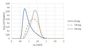
Figure 9: Heave spectra for 12 knots ship speed with 90°, 135° and 180° wave headings.
