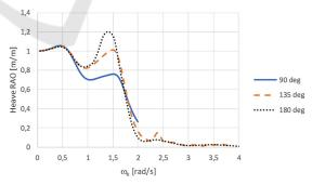
Figure 7: Heave RAOs for 12 knots ship speed with 90°, 135° and 180° wave headings.
