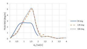
Figure 8: Pitch RAOs for 12 knots ship speed with 90°, 135° and 180° wave headings.
