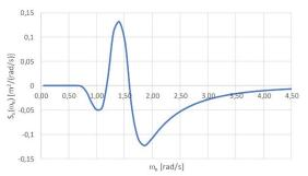
Figure 12: Relative motion spectrum at point I for 12 knots ship speed in head seas.
