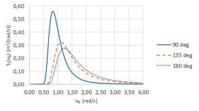
Figure 6: Encounter wave spectra for 12 knots ship speed with 90°, 135° and 180° wave headings.
