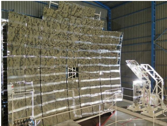
Figure 2: Parabolic concentrator, 45° inclined mirror and the test table of SF60 solar furnace.
