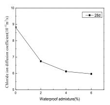
Fig 5:Effect of water-based organic silicon on chloride diffusion coefficient of concrete.
