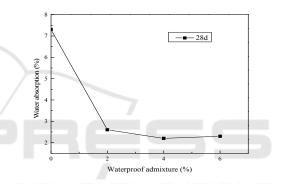
Fig 3:Effect of water-based organic silicon On water absorption of concrete.
