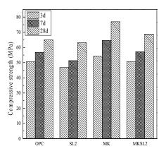
Fig2: Effect of modified metakaolin on compressive strength of concrete with water-based organic silicon.
