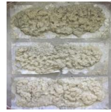
Figure 2: The measuring procedure of swelling capacity of SAPs by the tea bag method.
