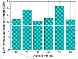
Figure 1Low temperature bending strength of asphalt mixture.
