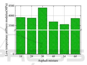
Figure 3Low temperature stiffness modulus of asphalt mixture
