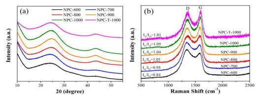
Figure 2. Powder XRD patterns and Raman spectra of six ZIF-derived nanoporous carbons.
