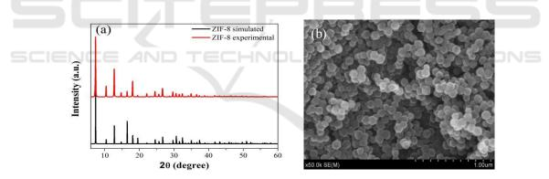
Figure 1. (a) XRD pattern and SEM image of ZIF-8.
