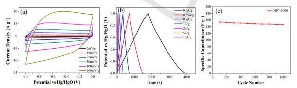
**Figure 6.** Capacitive performance of NPC-1000. (a) Cyclic voltammetry curves at different scan rates, (b) galvanostatic charge and discharge curves at different current densities, and (c) cycling stability at 5A g<sup>-1</sup>.
