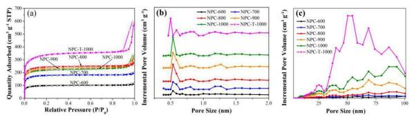
**Figure 4.** N<sub>2</sub> adsorption-desorption isotherms (a) and the corresponding pore size distributions of the ZIF-derived nanoporous carbons at different temperature, (b) micropore size distribution, (c) meso- and macropore size distribution.
