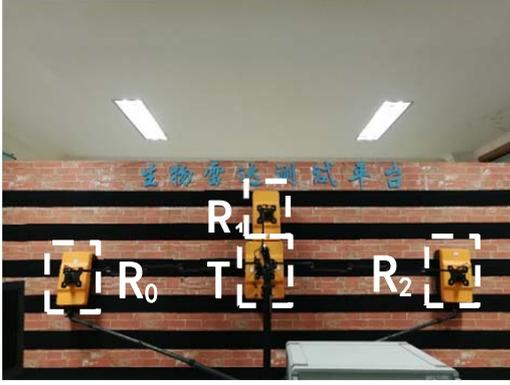
Figure 5: Antenna deployment in through-wall scenario.
