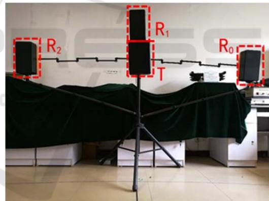
Figure 3: Antenna deployment in free-space scenario.
