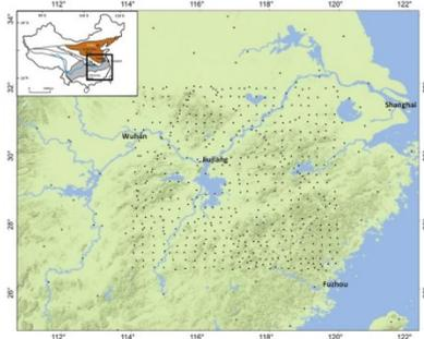
Figure 1: Map of study area and location of MT stations (The area of the work area is about 350 thousand square kilometres. A total of 525 wide-band magnetotelluric sounding stations were acquired.)
