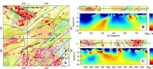
Figure 5: Vertical electrical characteristics of two profiles. (a) the position of two profiles AA' and BB'. (b) electrical characteristics of the West-East line BB'. (c) electrical characteristics of the South-North line AA'.
