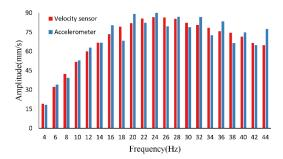
Figure 4: Peak-peak value contrast histogram between velocity sensor and accelerometer
