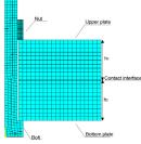
Figure 1: finite element model of the single bolted joint.
