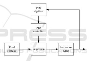
Fig.3 PID controller model for active suspension in simulink
