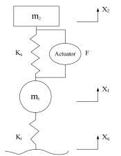
Figure 1:The quarter-vehicle body model of 2 DOEs.
