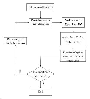
Figure 2: Optimization process of PID controller by PSO algorithm.
