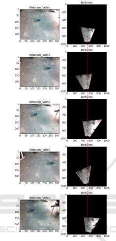
Figure 2: Fixed object IPM view with different Pepper Head Orientation (i.e: (yaw,pitch) = (36,0),(36,-10),(36,10),(36,-20),(36,20)).
