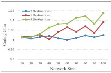
Figure 9: Coding Gain in Networks of Sparse Density.
