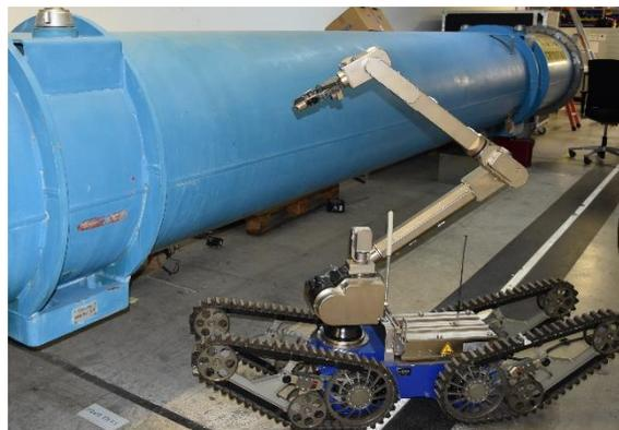
Figure 1: The teleoperated robot, Telex, during one of its maintenance procedures at CERN.
