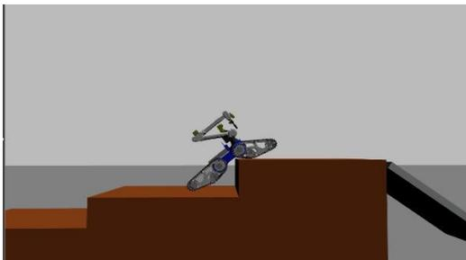
Figure 10: Telemax operated to climb up stairs by setting the flippers accordingly.
