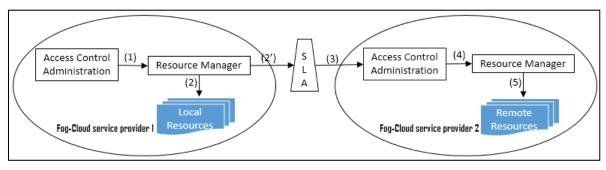
Figure 4: Distributed authorization process in the multi fog cloud.
